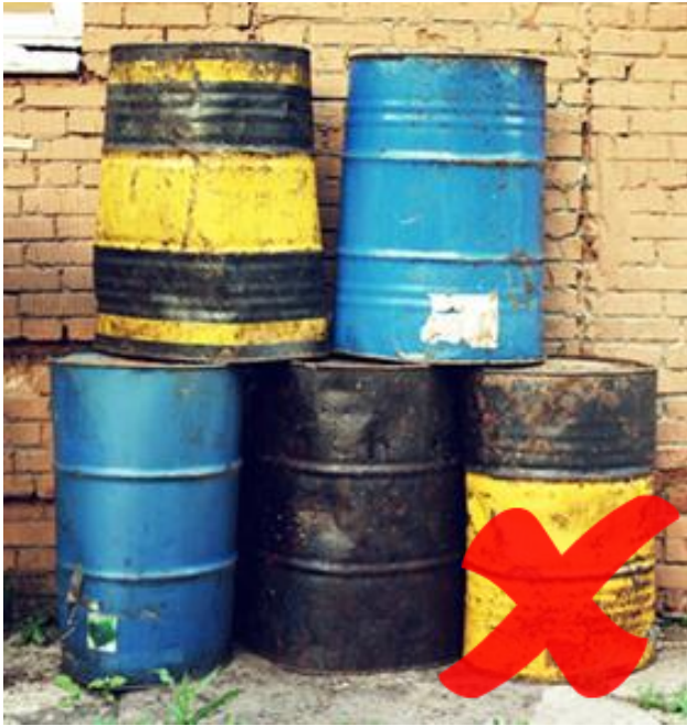
Bad practice: Liquid containers stored outside without secondary containment.
