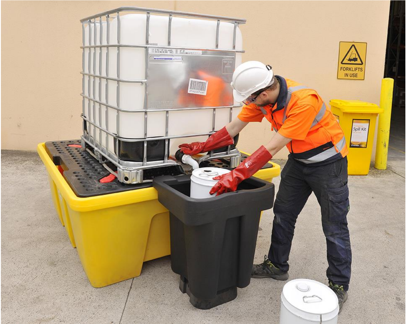
Figure 12: An intermediate bulk container (IBC) on a spill pallet with a dispensing unit attached. The spill pallet reduces the risk of leaks or spills from the IBC while the dispensing unit directs any potential spills during decanting into the sump.
