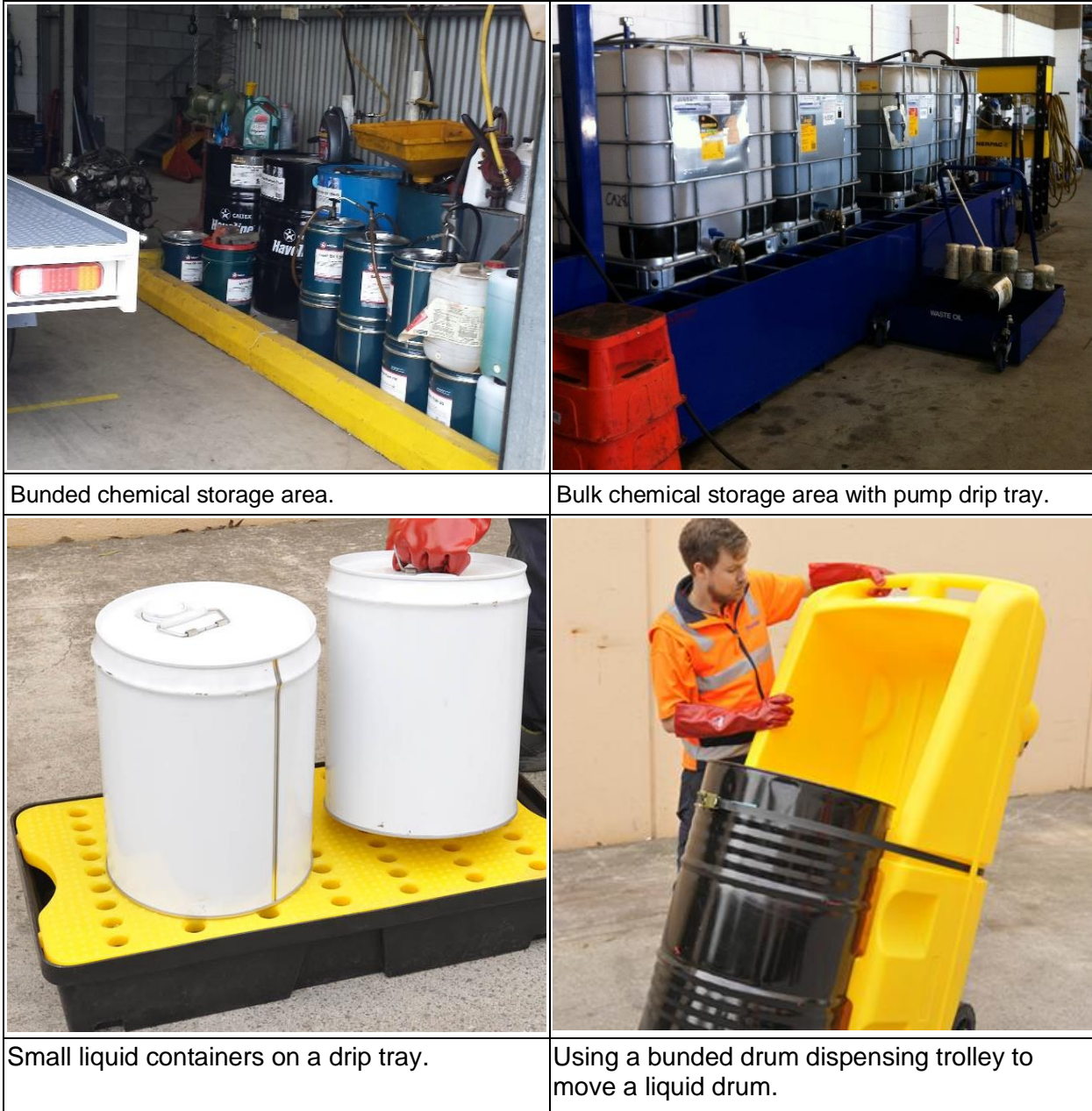
Figure 10: Some examples of secondary containment methods photographed from industry sites.
